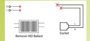
Connect directly to socket and install LED Lamp
